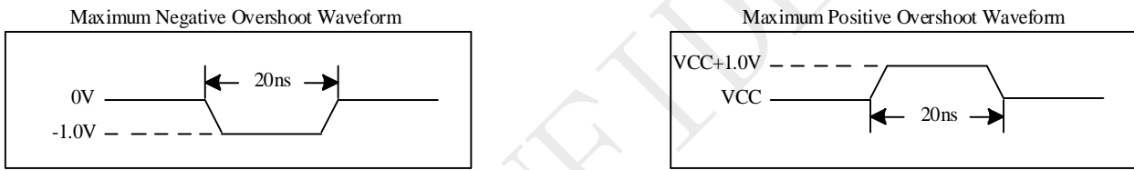
Figure 5-2 Input Test Waveforms and Measurement Level
